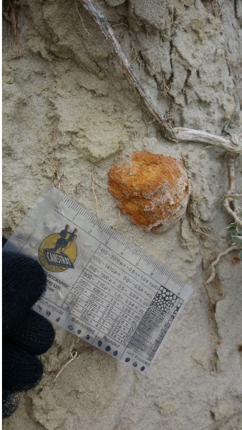
Figure 5 – Large concretions were observed in the upper unconsolidated sand unit in Transect 1 and Transect 2. Photo credit: Robert Nodge, 2015.
