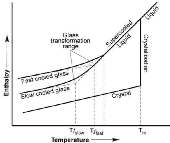
**Figure 4.6.1** – Diagram illustrating the effect of temperature on the enthalpy of a glass-forming melt (Grapes, 2011).
