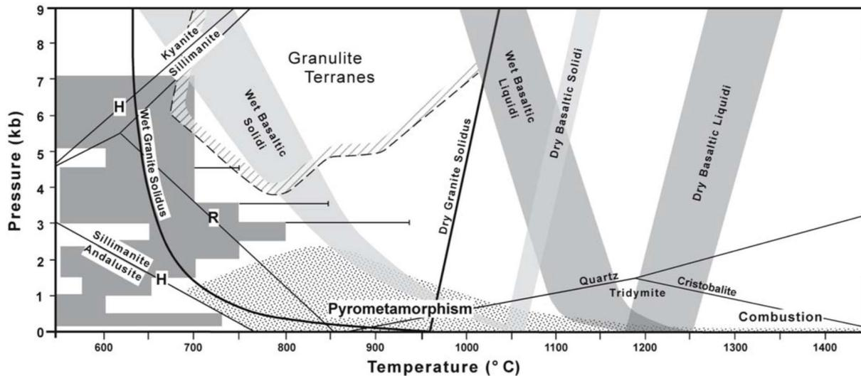
**Figure 2.2** – Diagram showing the sanidinite facies stability field and the relationship of sanidinite facies rocks (*stippled area*) to contact metamorphic and granulite facies rocks. (Grapes, 2011).
