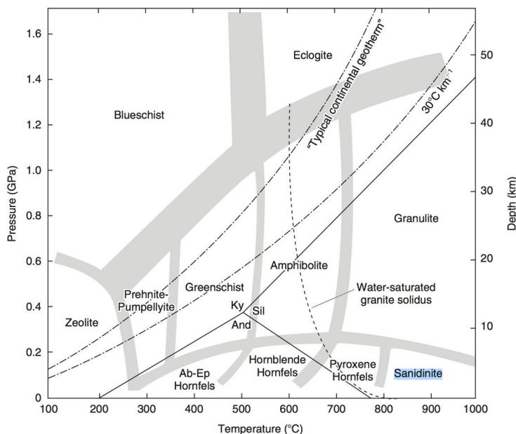
**Figure 2.1** – Metamorphic facies graph showing the stability range of each of the described facies. These are compared by both pressure (measured in GPa) and depth (in km) on the vertical axis and increasing temperature (in °C) on the horizontal axis. The occurrence of sanidinite facies is highlighted on the bottom right of the diagram (Kearey *et al.*, 2009).
